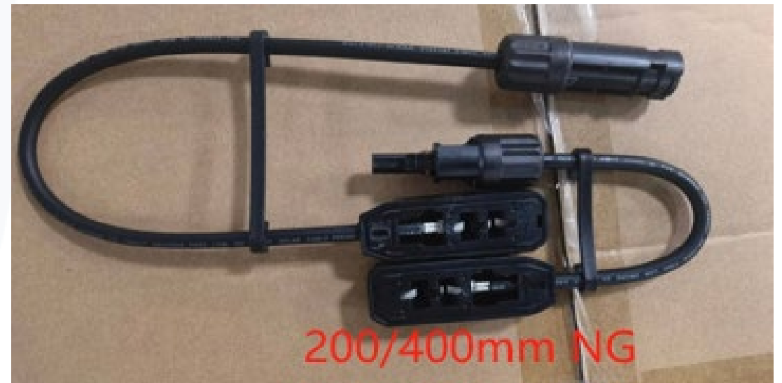
Incorrect junction box cable length of 200/400mm
