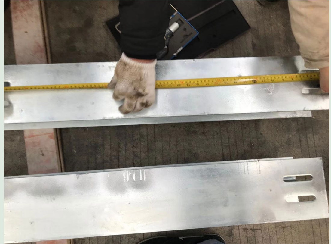
Dimension inspection for post:
