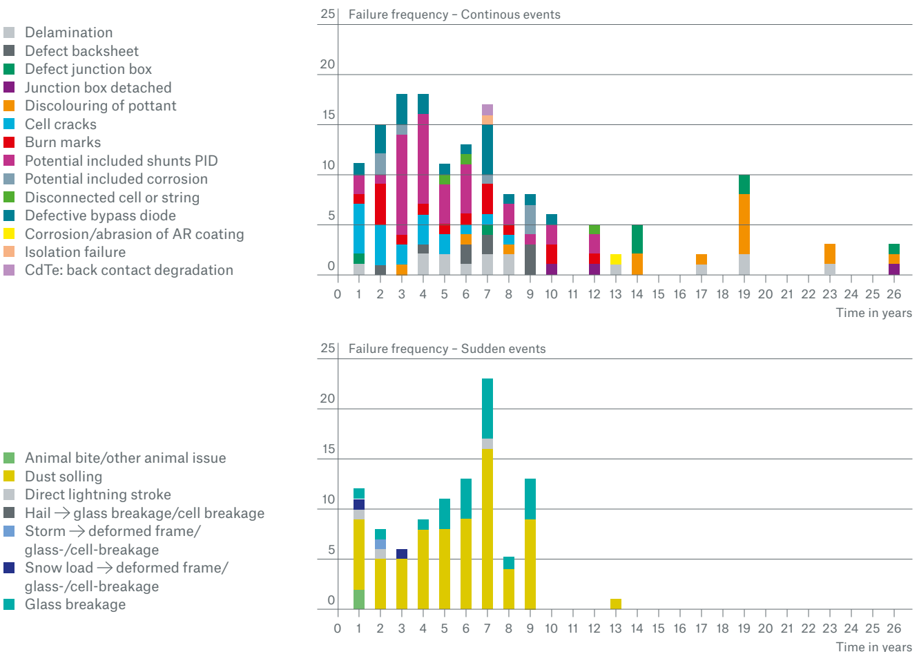
Figure 1: Failure frequency for PV module defects affecting system performance. The upper graph shows the failure frequency of PV modules with slow degradation over time and the lower graph shows the failure frequency for sudden events [Köntges2017].
