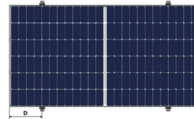
Installation of framed module with fixtures on long sides Beam perpendicular to long sides (clamp length \geq 50 mm)
